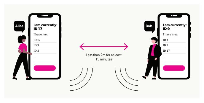
Schematic and simplified presentation of the functioning of the Corona tracing app.<sup>11</sup> Each phone will keep a "local" and anonymized record of all phones (carrying the app) with which it was in close proximity for longer than 15 minutes. The issued IDs are temporary but can be decrypted by the server.
